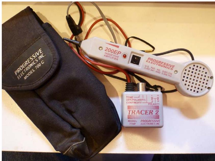
*A typical signal tracer set consisting of a tone generator/continuity tester (small box marked "Tracer 2") and signal tracer amplifier/'banana' (marked 200EP.)*
