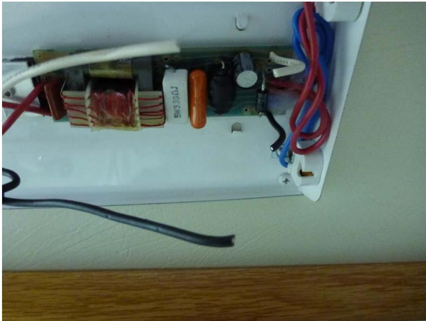
The 12-volts power wires from the vehicle 'ground' and power switch to the ballast circuit are the ones we'll cut and use for the LED strips.
