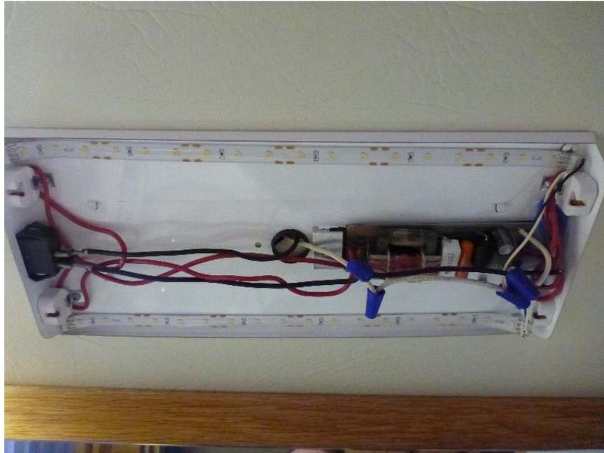
LED strips secured inside the fixture.
