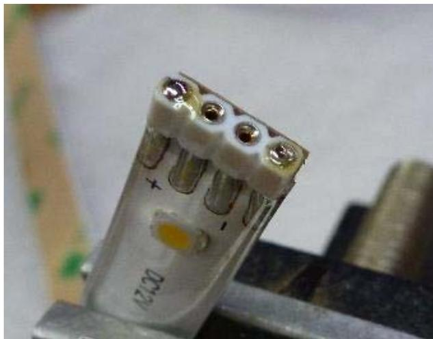
Solder 'tin' two connection points at the end of the LED strip. Note + and -.
