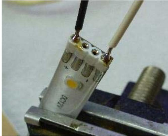
Attach 5 inches of wire to each LED strip contact point. Best if the wire color matches the wires/polarity of the fixture/ballast circuit.
